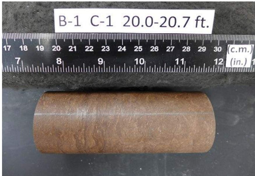
After cutting and grinding
