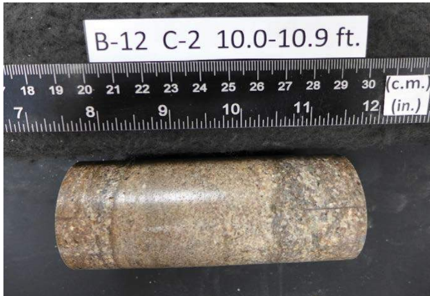
After cutting and grinding
