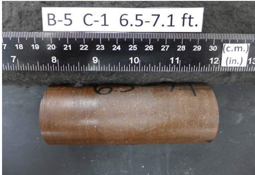
After cutting and grinding
