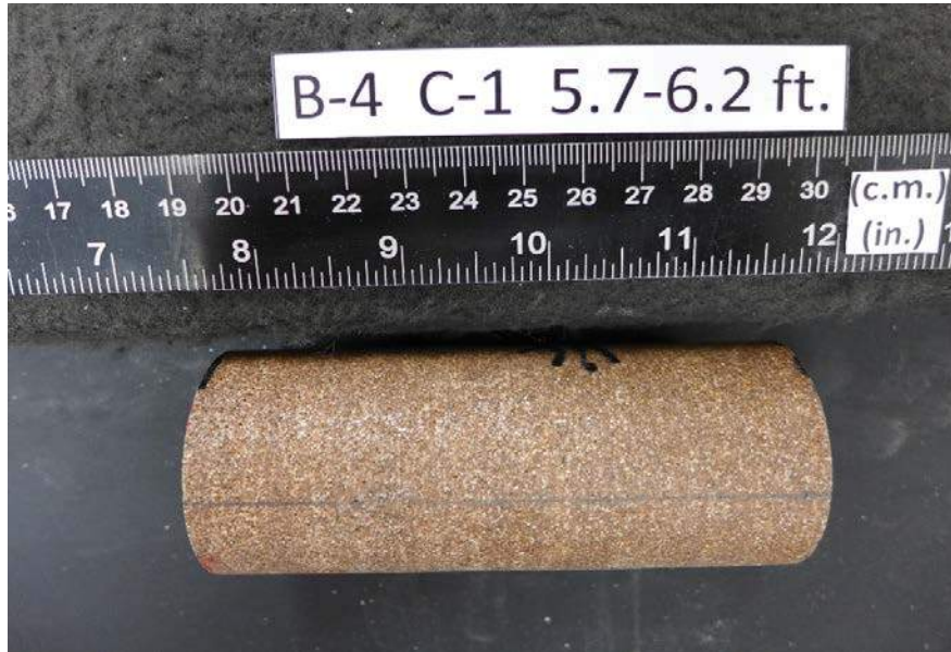
After cutting and grinding
