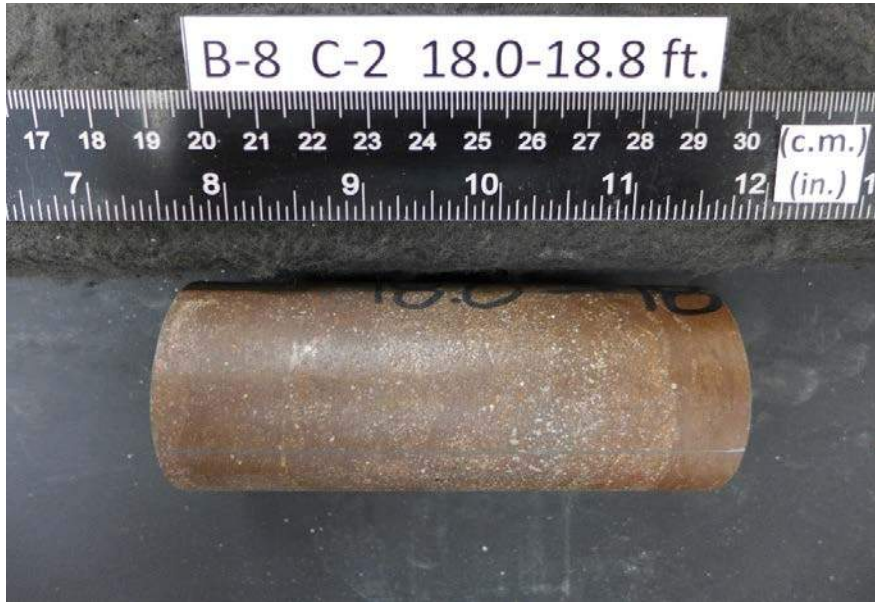
After cutting and grinding
