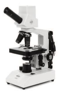
With built-in 3.0 mega pixel camera (1280 x 1024), this monocular digital microscope comes standard with 4XD, 10XD, sealed 40XRD objectives (sealed 100XRD is optional), 18mm eyepiece, separate coarse and fine focusing, built-in mechanical stage, substage 1.25 Abbe condenser and variable LED illumination. Motic Images Plus software and calibration slides included.
